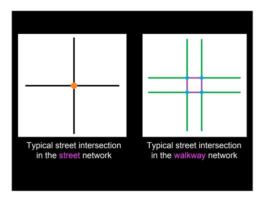
In the street network model the nodes are intersections and the arcs are the roadway segments. In the walkway network model the nodes are street corners and the arcs represent both sidewalk segments, in green, and crosswalk segments, in purple.
