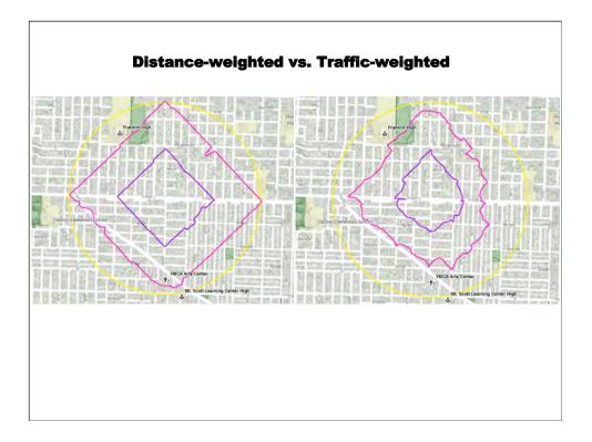
Here you see an example of the kind of side-by-side walkshed comparison that the walkway network model team created for each proposed transit station. On the left are the half-mile and quarter-mile walksheds with walking constrained to a network weighted only by distance. These distance-weighted walkshed diagrams can help illuminate where connectivity might be improved using cut-throughs.
