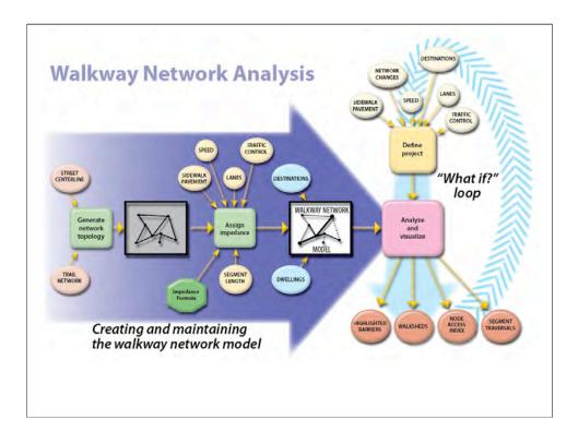
The walkway network analysis process has two parts: creating and maintaining the walkway network model, indicated by the big dark blue arrow, and the "what if?" loop, represented by the light blue arrows, where you can try out and compare different improvements.
