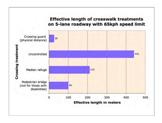
Let's compare the relative effective distances for these different crossing treatments. The effect of the median refuge island on effective distance is accounted for by summing the sub-crossings, which substantially reduces the effect of the multi-lane term for the total crossing. For the pedestrian bridge, we estimated the effective distance as twenty-four times the vertical gain, plus the actual distance to cross.
