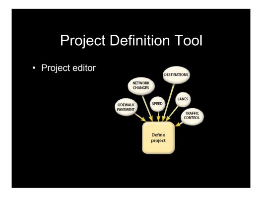
Once we're able to run analysis, we're ready to try out projects. A project in the model can be thought of simply as a new set of impedance values. These new impedance values reflect proposed changes to the environment such as lowering the speed limit, adding traffic control, paving sidewalks, or adding shortcuts.
