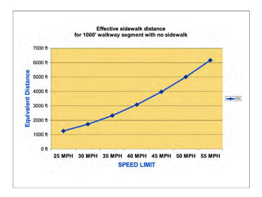
In the case of sidewalk segments with incomplete sidewalk paving, we've proposed that effective length is related to the speed of traffic on the associated street segment, and...
