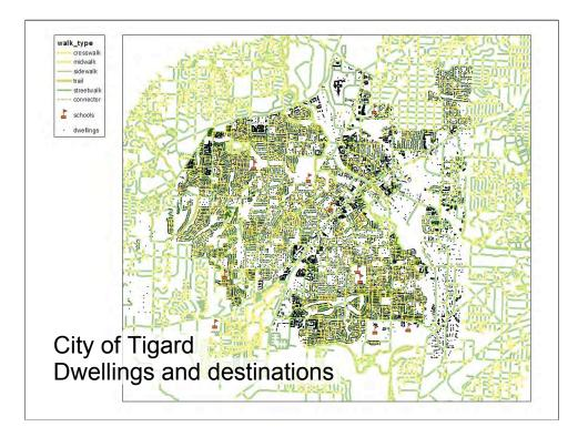
To analyze the network, trips must be routed from origins to destinations. In the walkway network model, dwellings are the origins and many different classes of destination can be loaded, such as schools, shown here, or grocery stores, or parks.
