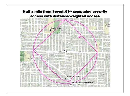
Since pedestrians don't fly, the walkshed must be constrained to the network, as shown by the inner line here. For a perfect street grid, constraining trips to the network produces a diamond-shaped walkshed. Here you can see how slight anomalies in the grid affect the walkshed shape.
