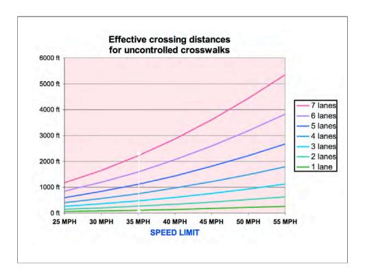
The shape of the effective distance versus speed limit curve is a parabola; in this case, it is also a power function. This shape is proposed because it is the shape of the stopping distance versus speed curve for motor vehicles.
