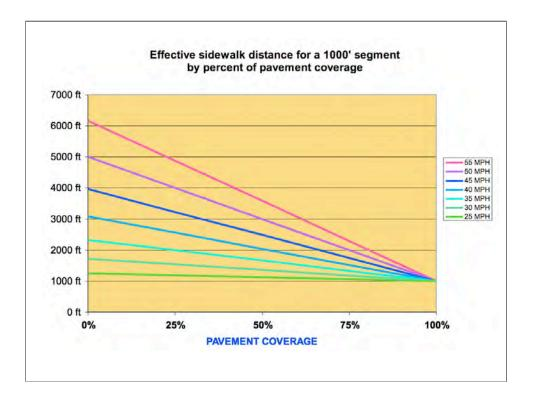
... also proportional to the percent of pavement coverage. Here the proposed curve fitting parameters are chosen so that an unpaved walkway segment on a 25 mph (40kmh) street has an effective length of one and a quarter times its geographic length, and an unpaved walkway segment on a 50 mph (80kmh) highway has an effective length five times its geographic length.
