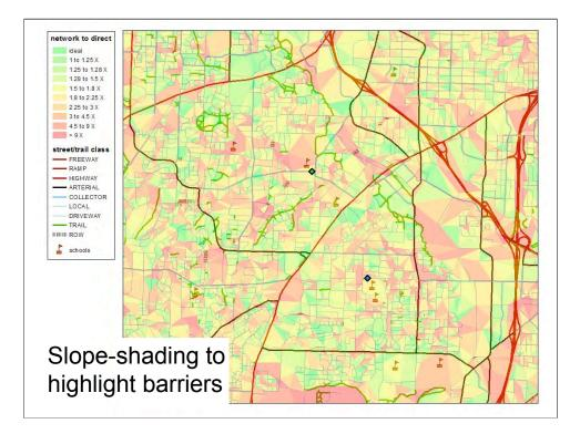
Another way to visualize analysis results is to use slope shading to highlight barriers. Here we're back to Tigard, looking at access to the two middle schools. Green areas represent places where the ratio of effective distance to crow fly distance is one, or close to one. In the red areas the effective distance is nine times the crow fly distance, or more.
