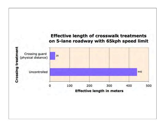
Although the actual distance to cross is only about 26 meters, the effective distance in the walkway network model is 440 meters.
