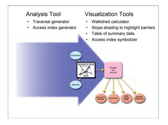
The core of the analysis is a routing engine that can calculate tens of thousands of lowest impedance paths in a minute. It calculates the lowest impedance path from each dwelling in the data set to its closest destination in a class of destinations.
