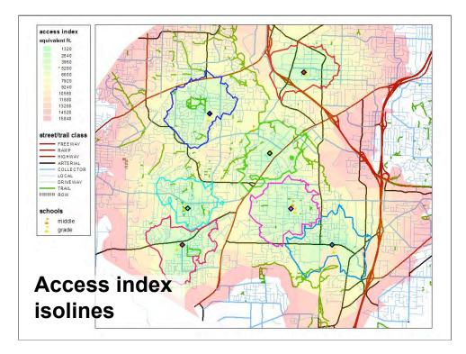
The access index is a value for each node that represents the sum of the impedance values for all the segments on the lowest impedance path from that node to the nearest destination of a class -- in this case, the nearest school. This shaded map shows areas colored according to their access index values, with isolines representing the effective one-mile walksheds around each school.
