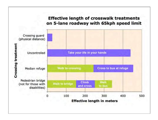
Suppose you are trying to reach any bus stop on the opposite side. Is it worth going out of your way to an easier crossing? Here's how the options stack up, including walking along the street from where you started.
